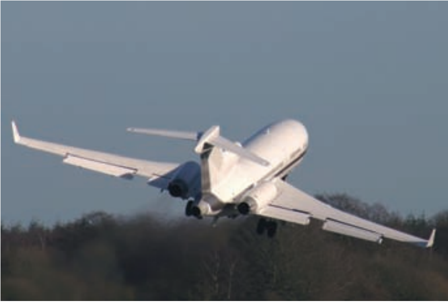
The first use of a winglet on commercial transport aircraft was the Valsan winglet (now Quiet Wing Corp) on the 727.
