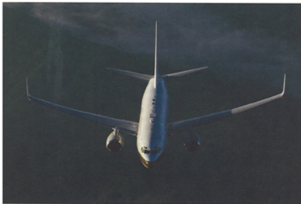
Figure 2.1 Boeing business jet with Aviation Partners Blended Winglets
