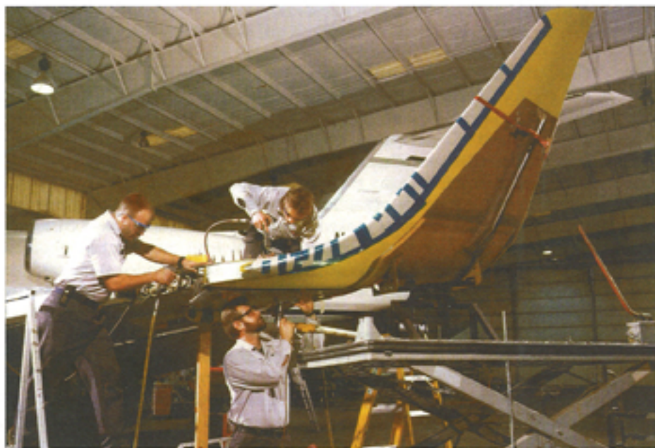
Blended Winglet being installed on a Gulfstream
