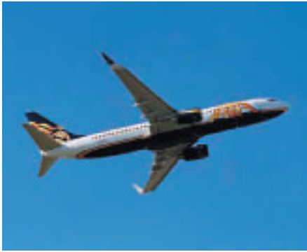
ATA Airlines is among the airlines operating B737-800s equipped with APB winglets.
