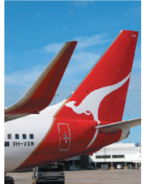
Qantas' evaluation of the B737-800 initially considered an east-coast network and the use of blended winglets was found to be beneficial both to range and fuel burn.
