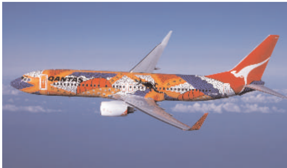
Australian carrier Qantas Airways has APB winglets installed on its B737-800.
