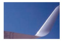
carbon monoxide and nitrous oxide emissions by 4 per cent and 5 per cent respectively while decreasing the take-off noise footprint by 6.5 per cent. Thanks to improved wing efficiency and reduced noise footprints, many Blended Winglet-equipped operators in Europe have been able to decrease operating fees and noise surcharges by opting for lower-thrust engines and lower max take-off weight.
